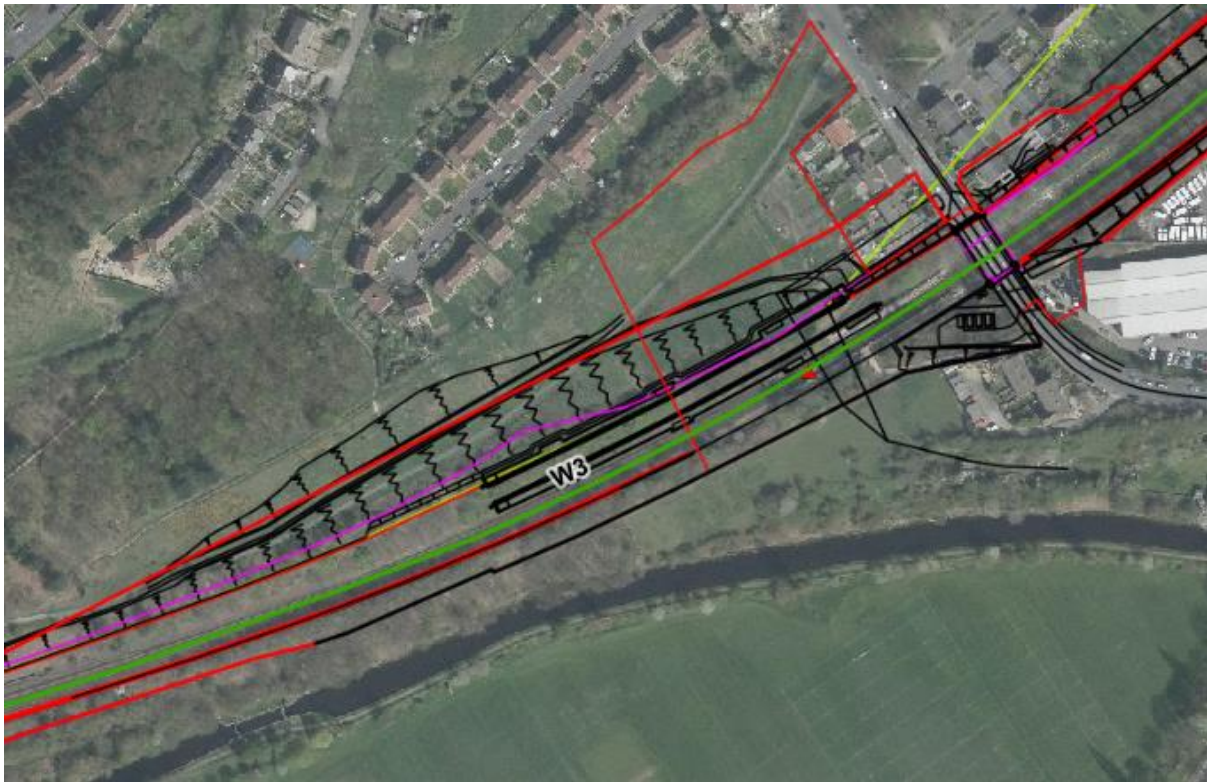
Figure 1: Embankment design, Deighton Station
